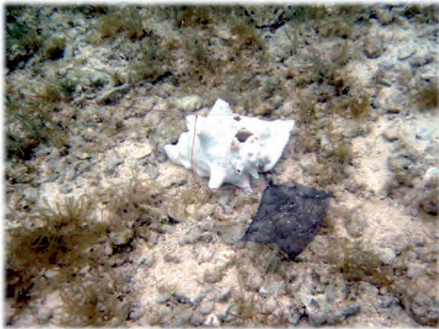
Figure 18. Artificial substrate. A 750 cm 2 piece of window screen fabric is used as “artificial seaweed” to collect Gambierdiscus and Ostreopsis cells. This artificial substrate is shown attached to a conch shell with monofilament line in a bed of Acanthophora (NOAA).
