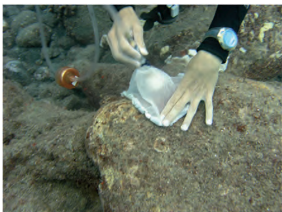
Figure 17. Dino-Vac, the suction-operated sampling device used to collect epiphytes from turf algal substrates (pictures from Parsons et al., 2010, with permission).
