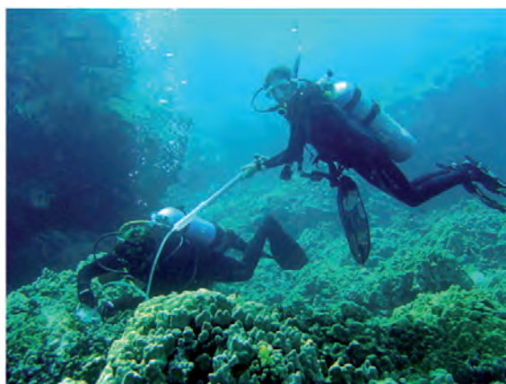
Figure 17. Dino-Vac, the suction-operated sampling device used to collect epiphytes from turf algal substrates (pictures from Parsons et al., 2010, with permission).
