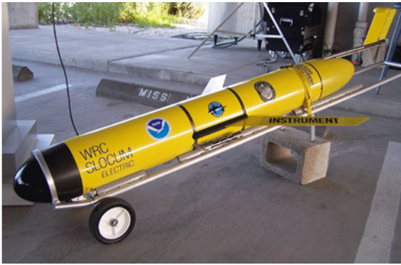
The Slocum Glider AUV with “Brevebuster,” an automated sensor for detecting Karenia brevis . Photo: Gary Kirkpatrick, Mote Marine Laboratory
